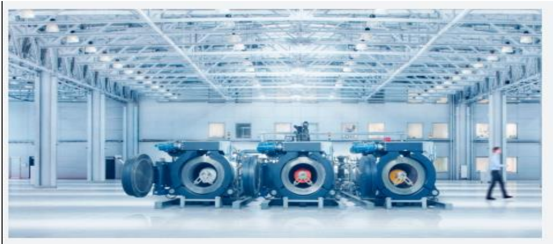
Figure (4): Waterless Dyeing Technology Units. Source : (Siraj Tahir, Martin r, & Tristan , 2019, p. 22)
